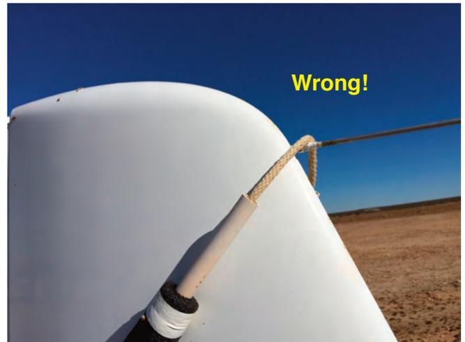
Wrong, on so many levels. Rudder lock should not hang down from the total energy probe. This lightweight fitting is not designed to carry any type of load such as this, particularly if the winds are strong. Installed in this manner, the lock does not prevent the rudder from flopping back and forth in the wind. Wind gust of 30 - 40 mph had been recorded in the week before.
