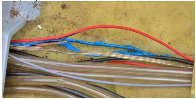
"Once that was done I carefully inspected everything. The ground wires, obviously, were unusable. However, the other wires were not damaged other than three spots on the positive wires. Also, there was a melted spot on the pitot tube. I couldn't tell if the pitot tube had melted completely through, so I covered that area with some shrink tubing. I also did the same for the three spots on the positive wires.
