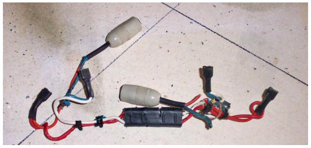
"Current equals Voltage times resistance – E=IxR. Manipulating, Current equals Voltage divided by resistance – I=E/R. The only resistance in the circuit created was in the copper wire and the internal resistance of the batteries, practically 0 ohms.
